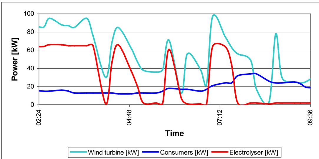
Figure 4: Example of operation. During the period one can see high wind modes with H<sub>2</sub>-production in the electrolyser.
