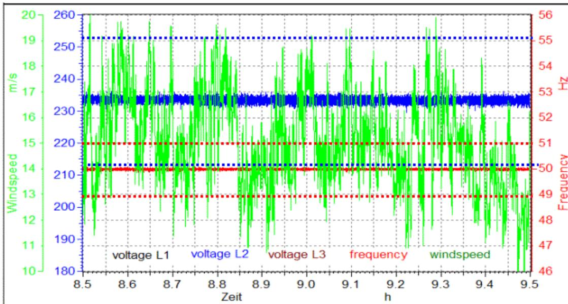
Figure 7: Grid quality measured (1 hour) in the stand alone system. Both frequency (red) and voltage (three phases – blue, brown and black) is well within the required norm EN 50160 (limits – dotted lines). Wind speed measured during this period shown in green.
