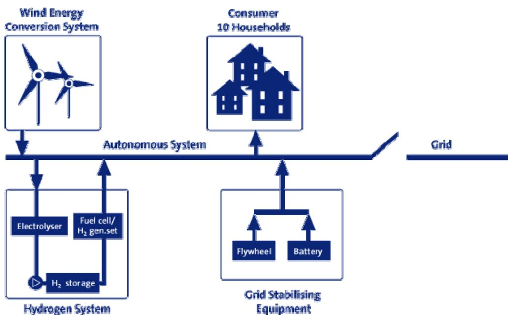
Figure 1 Illustration of the Utsira stand-alone wind-hydrogen energy system.
