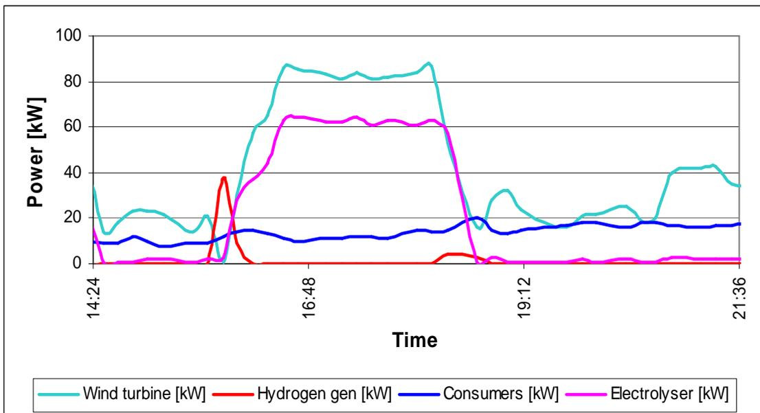
Figure 5: Example of operation. During the period one can see both the high wind mode with H<sub>2</sub>-production in the electrolyser and the low wind mode with the H<sub>2</sub>-engine balancing the consumers demand.
