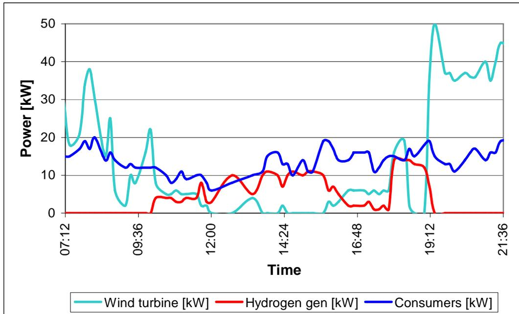
Figure 3 Example of operation. During the period one can see that the wind power decreases and cannot supply the demand. In this period the H<sub>2</sub>-engine is started and is balancing the load.
