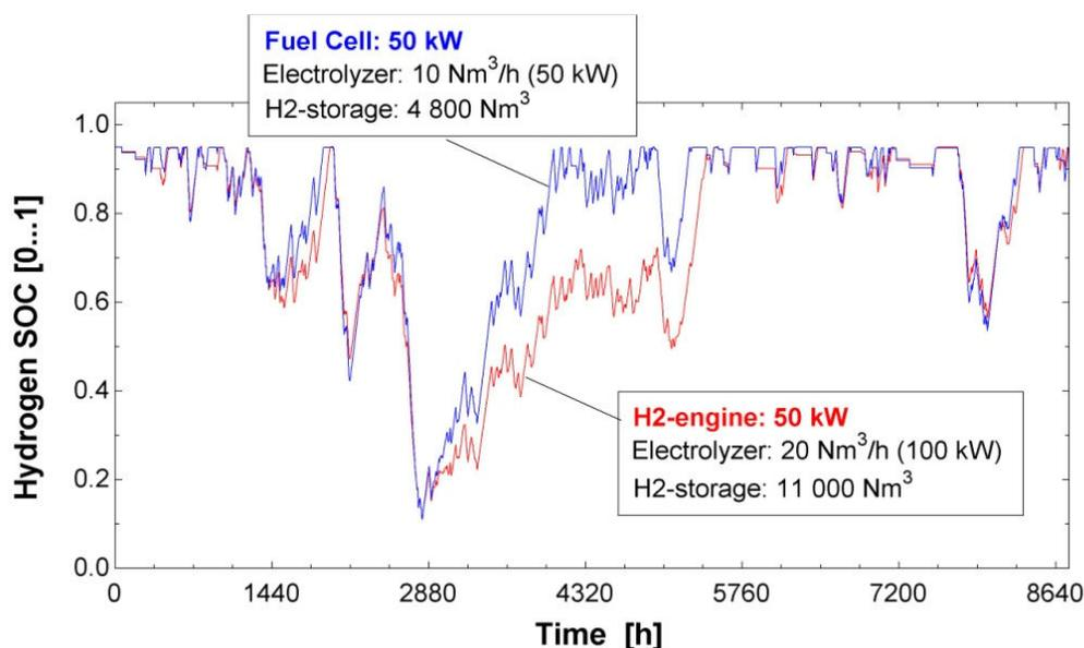
Figure 7: Comparison of two alternative system configurations: fuel cell versus hydrogen engine
