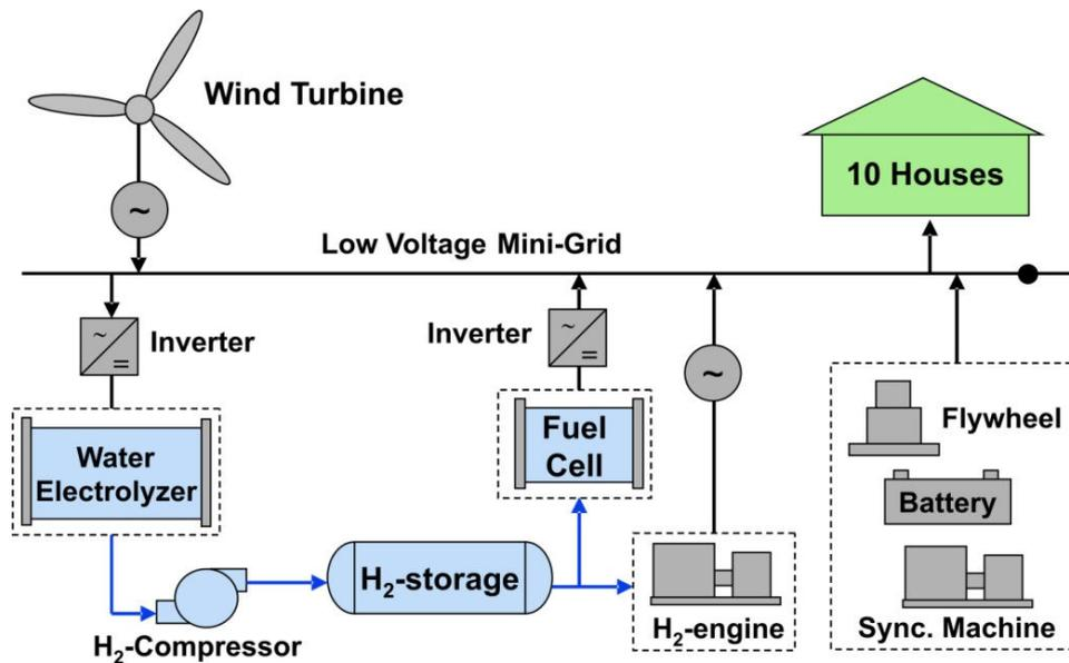
Figure 2: The energy system installed at Utsira
