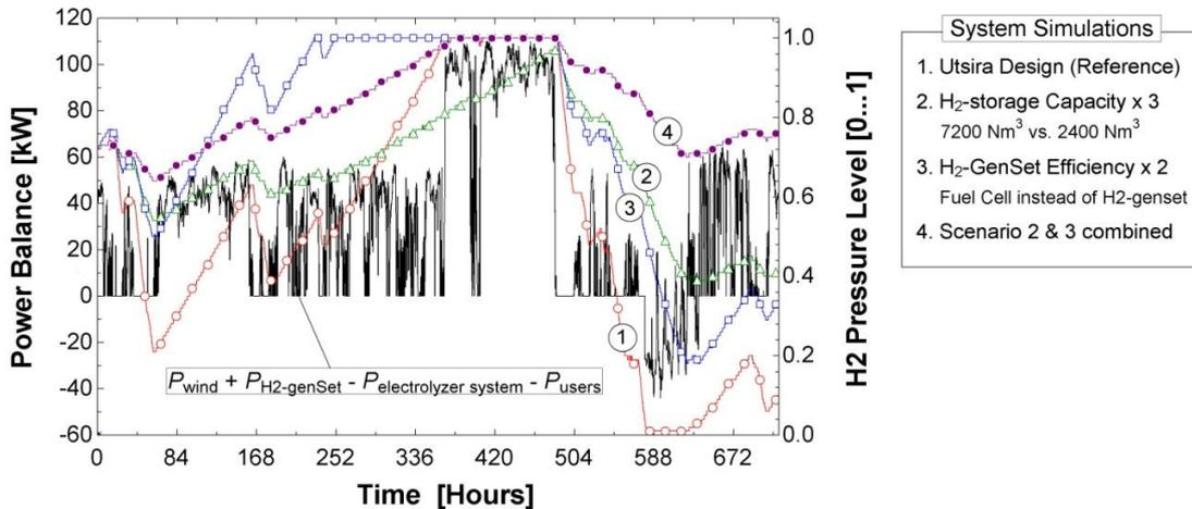
Figure 6: Wind/hydrogen system simulation results for (input data from Utsira, March 2007).
