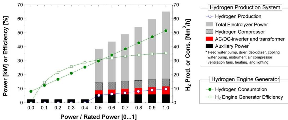
Figure 5: Modelling of electrolyzer system and hydrogen engine
